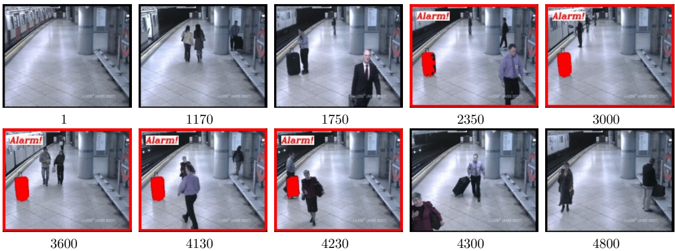
Figure 6. Test sequence AB-easy from AVSS 2007 (Courtesy of i-LIDS ). The alarm sets of immediately when the item is removed even though the luggage was stationary 2000 frames ( 180 \times 144 ).
