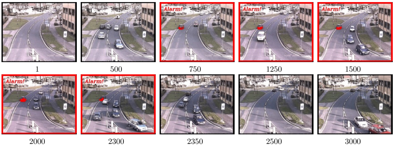
Figure 5. Test sequence PV-medium from AVSS 2007 (Courtesy of i-LIDS ). A challenge in this video is the rapidly changing illumination conditions that cause dark shadows.
