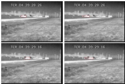
Fig. 2. Left column: Results of our tracker. Right column: the tracker using a naive template update strategy which updates template at each frame.
