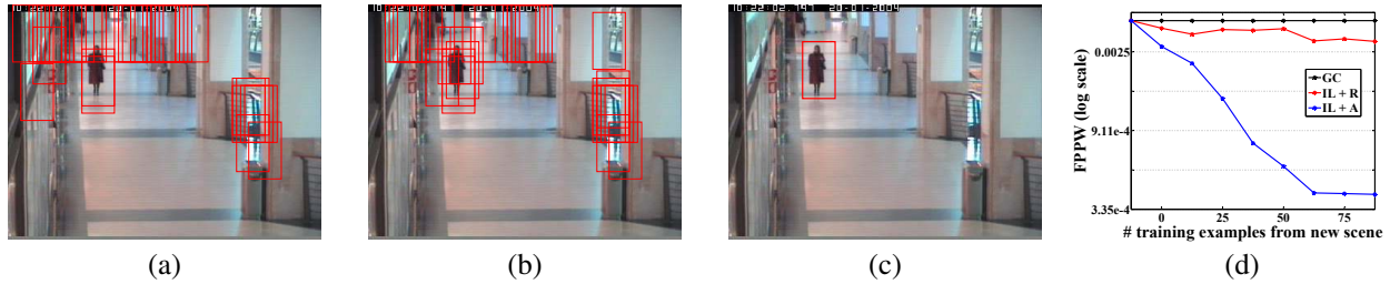
Figure 3. Sample results with 75 training examples from CAVIAR, (a) Generic classifier, (b) Incremental learning with random selection, (c) Incremental learning with active selection. (d) FPPW values of different methods with varying number of training examples on VID.
