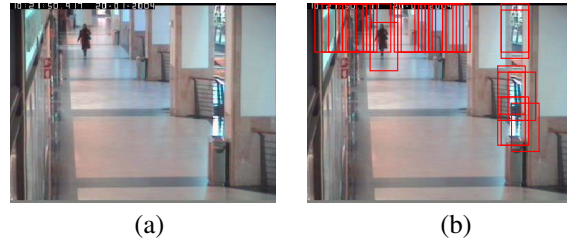
Figure 1. (a) Original frame. (b) Output of a human detector trained on the INRIA dataset.
