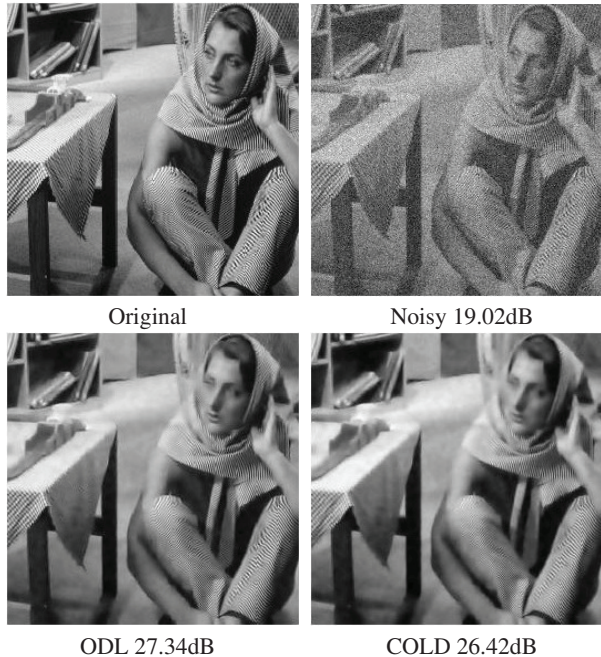
Fig. 4. Image denoising samples. COLD only needs less than 20% of the computations required by ODL, as seen in Table 2.
