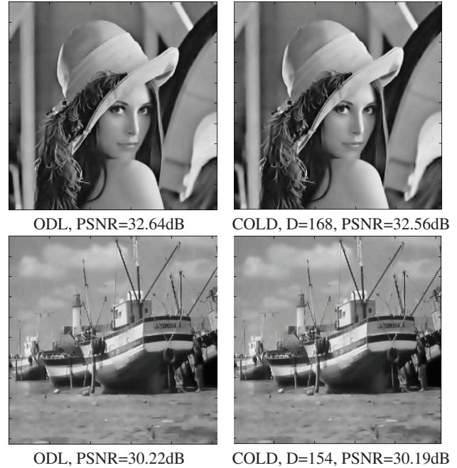
Fig. 5. Images on the left are the reconstruction obtained from ODL and the one on the right is the reconstruction using COLD. D denotes the dictionary size.
