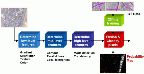
Figure 2: Flow diagram of road likelihood computation
