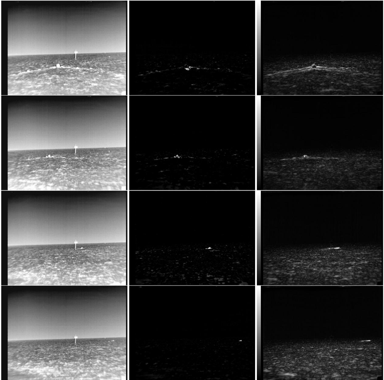
Figure 5: **Left:** Select frames from the sequence. **Center:** The distance transformed images that are generated by the multi-modal Gaussian background algorithm. **Right:** Corresponding images created by the 64-point FFT Waviz algorithm. Bright means novel. Frames are individually normalized.
