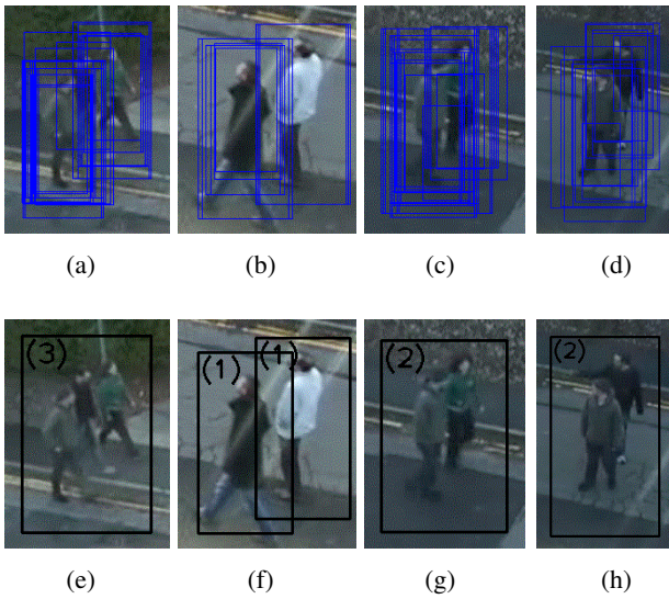
Figure 4: HOG detections (first row) and clustering results with number of people (second row) for BEHAVE dataset
