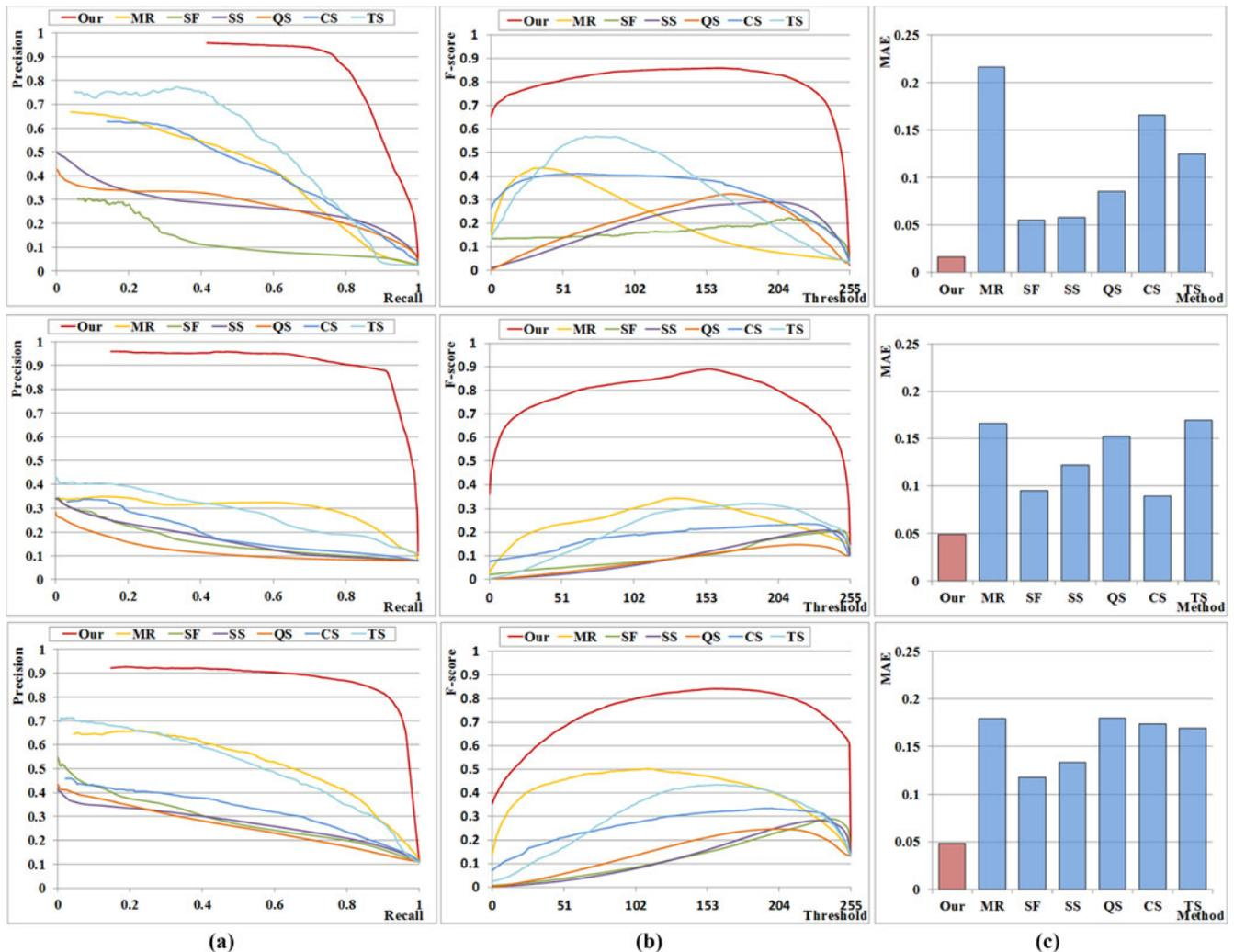
Fig. 6. Comparison of saliency detection methods using SegTrack [59] (*top*), extended SegTrack [60] (*middle*) and FBMS [1] (*bottom*) with pixel-level ground-truth: (a) average precision recall curve by segmenting saliency maps using fixed thresholds, (b) F-score, (c) average MAE.
