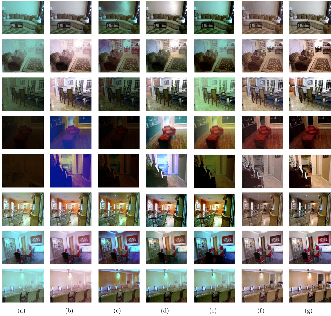
Fig. 5. Qualitative comparisons for samples from test set. (a) Raw underwater images. (b) Results of RED [21]. (c) Results of UDCP [22]. (d) Results of ODM [25]. (e) Results of UIBLA [26]. (f) Our results. (g) Ground truth. The types of underwater images in the first column from top to bottom are Type-1, Type-3, Type-5, Type-7, Type-9, Type-I, Type-II, and Type-III. Our method removes the light absorption effects and recovers the original colors without any artifacts.
