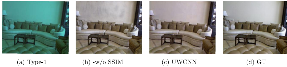
Fig. 11. An example of the importance of SSIM loss. (a) An underwater image with Type-1 degradation. (b) Result produced by UWCNN-w/o SSIM, which is a failure case since the background is not similar to the GT. (c) Result produced by our UWCNN. (d) Ground truth.
