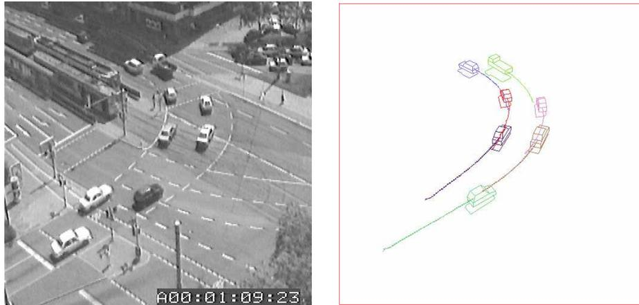
Figure 2.11: Cars are found, modeled and tracked using models .
